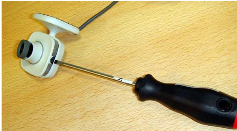
Fig. 3 - Take a flat head screwdriver and gently pry the case apart
